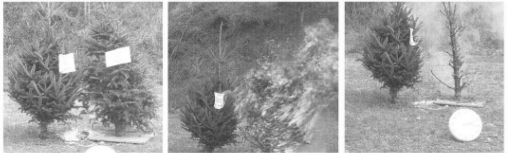
Figure 1. A fresh tree displayed in water (left) versus a dry tree displayed without water (right).
